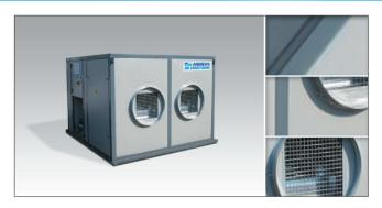
150 kW air handling unit can connect to your existing chilled water circuit or to an Andrews packaged water chiller, heat pump or boiler. These units are fitted with fan speed controllers and internal condensate pumps.
