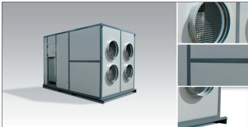
300 kW air handling unit can connect to your existing chilled water circuit or to an Andrews packaged water chiller, heat pump or boiler. These units are fitted with an internal condensate pump. A full range of ancillaries are available, including insulated flexible duct, plenum chambers, extraction fans and condensate hose.
