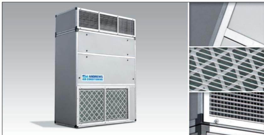
50 kW air handling unit can connect to your existing chilled water circuit or to an Andrews packaged water chiller, heat pump or boiler. These units are fitted with fan speed controllers and internal condensate pumps.
