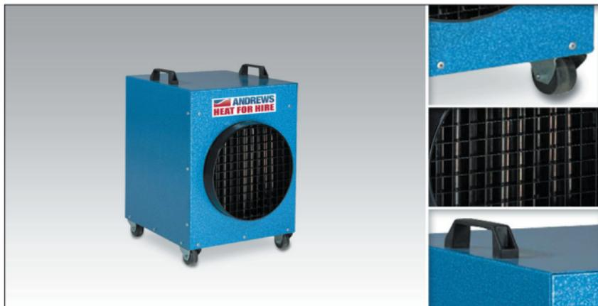
The DE95 is a very efficient electric fan heater and is available as a 415 volt 3 ph version only. The unit has three settings, 10 kW, 15 kW or 20 kW and can either be hard wired or supplied with a short cable tail and suitable plug. For automatic operation, the DE95 can be used in conjunction with the T32 control thermostat.
