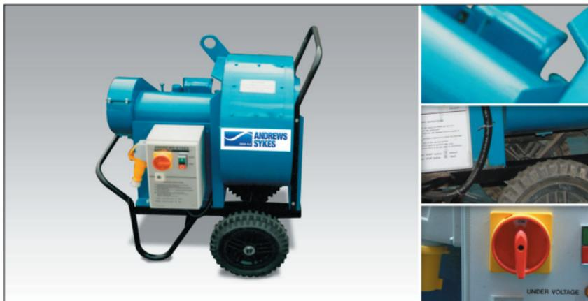
The FV300 ventilation/extraction fan is a robust high powered fan, used with ducting for the removal of dangerous fumes, dust particles and vapours. The FV300 has a maximum-ducted length of 40mtr and can be linked to heaters, boilers and chillers to distribute warm or cool air over large areas. The FV300 runs on 110 volt power supply.
