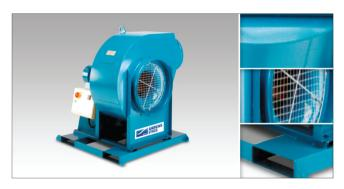
The FV900 ventilation/extraction fan is a robust high powered fan, used with ducting for the removal of dangerous fumes, dust particles and vapours. The FV900 has a maximum-ducted length of 40 metres and can be linked to heaters, boilers and chillers to distribute warm or cool air over large areas. This unit requires a 415 volt 3 ph power supply.
