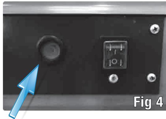
If the heater is allowed to run out of fuel the lockout light will illuminate. Replenish fuel supply and press reset button.
