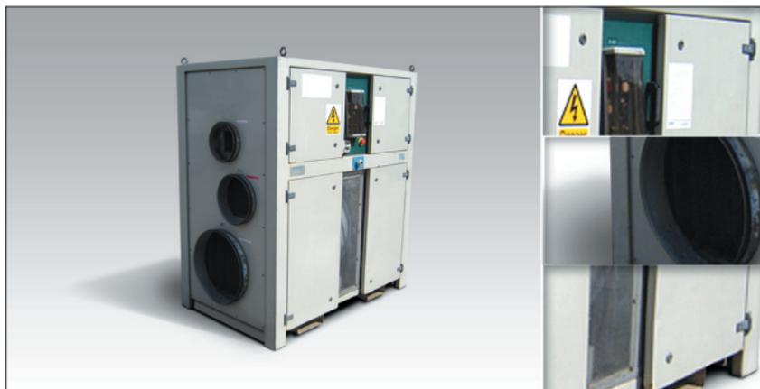
The KT6000 desiccant dehumidifier, is best used where the work is being carried out at very low temperatures and very low relative humidity is required. The KT6000 desiccant dryer is more efficient than refrigerant dryers at about  $-5^{\circ}\text{C}$ . This unit requires a 415 volt 3 ph power supply.
