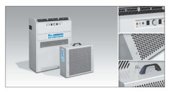
The PAC15, is a stylish water - cooled 'Split' portable air conditioner. Split means there are two parts to the system, the room unit and the external condenser unit, The two are connected by a length of flexible line. With the PAC15 the smaller condenser unit can be placed up to 30 metres from the room unit.
