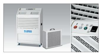
The PAC22 is one of our larger and more powerful stylish water - cooled 'Split' portable air conditioners. Split means there are two parts to the system, the room unit and the external condenser unit, The two are connected by a length of flexible line. With the PAC22 the smaller condenser unit can be placed up to 30 metres from the room unit.
