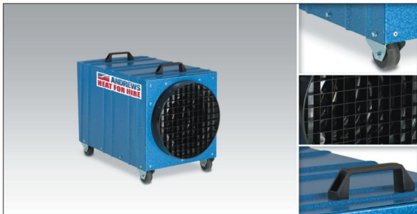
The DE65 is a very efficient electric fan heater and is available as a 415 volt 3 ph version only. The unit has three settings, 6.5 kW, 9.5 kW or 13 kW and can either be hard wired or supplied with a short cable tail and suitable plug. For automatic operation, the DE65 can be used in conjunction with the T32 control thermostat.
