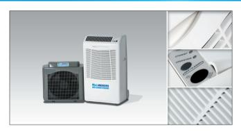
The PAC14 is a stylish refrigerant - 'Split' portable air conditioner. Split means there are two parts to the system, the room unit and the external condenser unit, the two are connected by a length of flexible hose. With the PAC14 Series 4 QC the smaller condenser unit can be placed up to 4 metres from the room unit.
